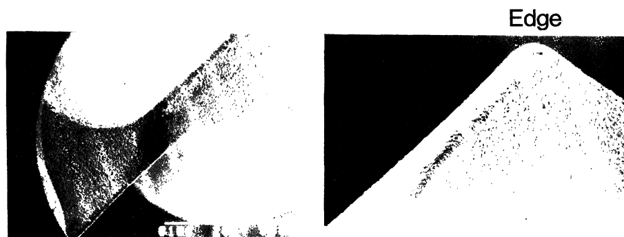
Figure 8. Microdrill in situ coated with CVD diamond (Asahi Diamond Industrial).
