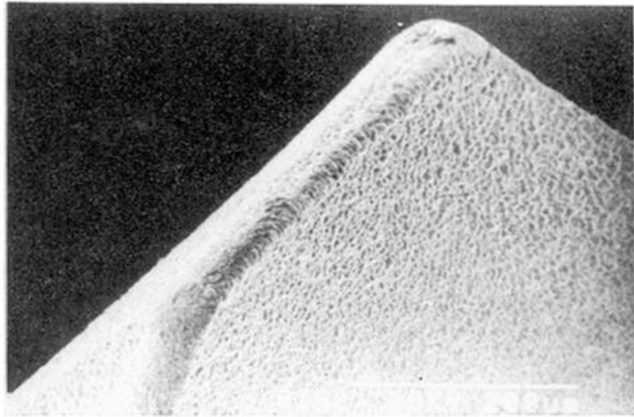
Figure 8. Microdrill in situ coated with cvd diamond (Asahi Diamond Industrial).
